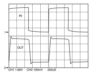
Figure 6: Square-Wave Modulation Linearity
