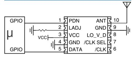
Figure 13: ES Series Transmitter Typical Application Circuit
