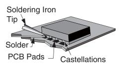
Figure 18: Soldering Technique
