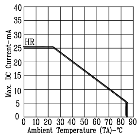
Fig5. MAX. ALLOWABLE DC CURRENT VS. AMBIENT TEMPERATURE.
