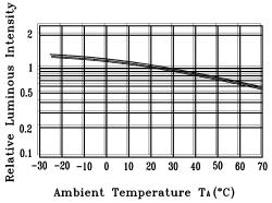
Fig.5 Luminous Intensity vs. **Ambient Temperature**
