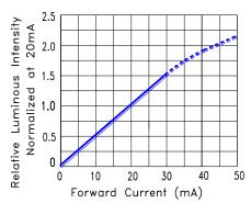
Fig.4 Relative Luminous Intensity vs. Forward Current
