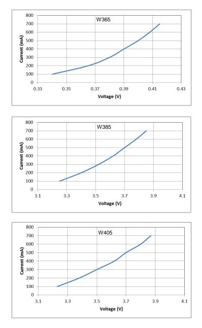
Fig 4. Forward Current vs. Forward Voltage of LTPL-C034UVHXXX
