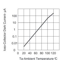
FIG.3 COLLECTOR DARK CURRENT VS AMBIENT TEMPERATURE
