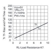
FIG.4 RISE AND FALL TIME VS LOAD RESISTANCE
