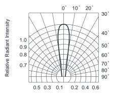
FIG.6 RADIATION DIAGRAM
