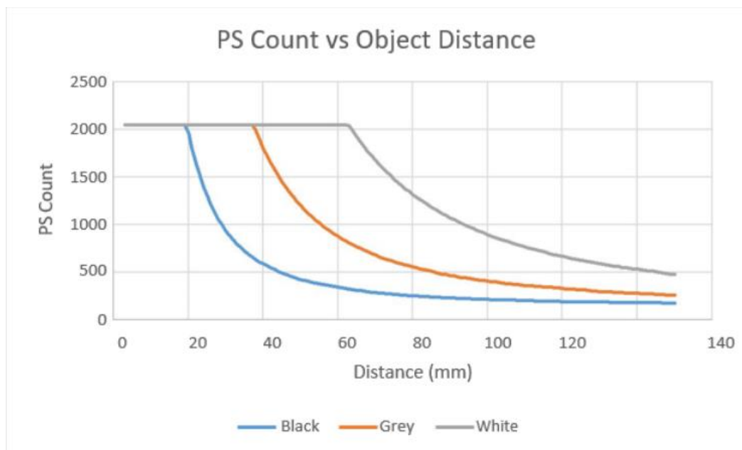
Figure 4.1: PS performance across distance VDD 1.8V, 104mA, 16pulses, with others in default settings.
