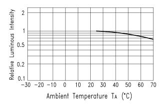
Fig.5 Luminous Intensity vs. Ambient Temperature
