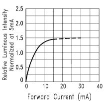
Fig.4 Relative Luminous Intensity vs. Forward Current
