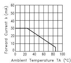
Fig.3 FORWARD CURRENT DERATING CURVE
