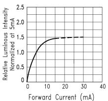
Fig.4 Relative Luminous Intensity vs. Forward Current
