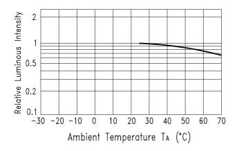
Fig.5 Luminous Intensity vs. Ambient Temperature
