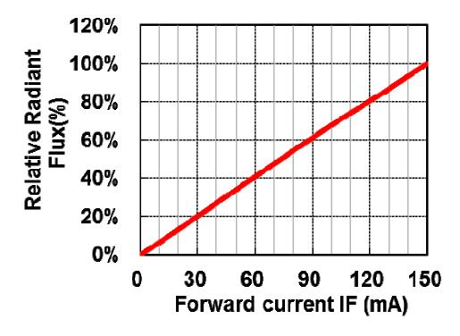
Fig.4. Forward Current vs. Relative Radiant Flux
