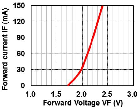
Fig3. Forward Current vs. Voltage
