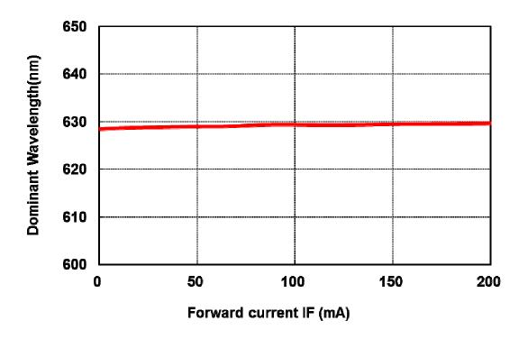
Fig.5. Forward Current vs. Dominant Wavelength
