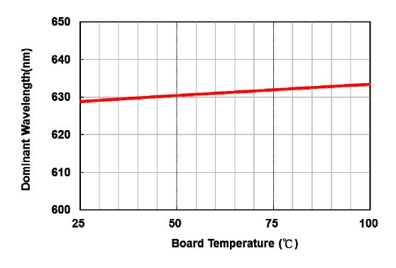
Fig.6. Board Temperature vs. Dominant Wavelength
