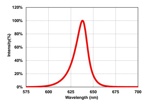
Fig1. Relative Spectrum of Emission
