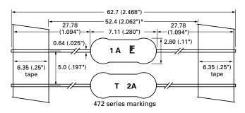
Coating Diameter (max): 0.5A-3.0A: 2.80mm 5.0A: 2.90mm
