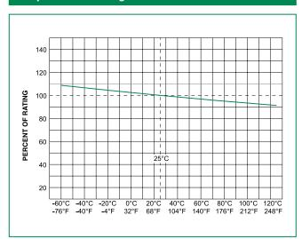
$\ensuremath{\text{NOTE}}$  : Derating depicted in this curve is in addition to the standard derating of 25% for continuous operation.
