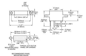
NOTE: The 20 ampere single pole holder is designed to accept all fuse ratings up to 20 amperes.
