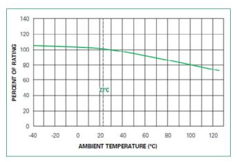
Note: 1. Rerating depicted in this curve is in addition to the standard derating of 25% for continuous operation.
