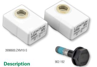
The Sealed M10 ZCASE fuse is designed to mount directly to a standard forklift battery to provide short circuit protection to the highest current circuits powering electric vehicles. Its placement on the battery eliminates the need for any unfused, high-current wires off of the battery-even the
