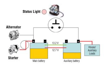
5 The engine is powering the alternator, and the starting battery has reached 13.2V. Only now does the Smart Battery Isolator reconnect, enabling the depleted auxiliary battery to be charged. By not reconnecting until the main battery is charged, the alternator is protected from excessive loads.
