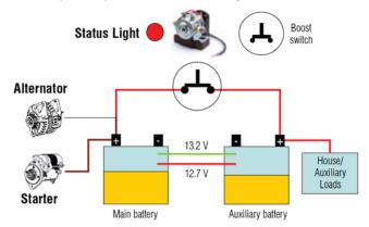
3 The alternator begins to charge the batteries. After one minute the Smart Battery Isolator reverts to the automatic mode. If the starting battery has not reached 13.2V, it isolates the batteries to reduce stress on the alternator. Once the main battery reaches 13.2V, it reconnects and charges the auxiliary battery.
