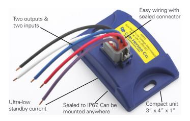
The FlexMod<sup>™</sup> family is a series of small, robust electronic modules. They have two inputs (one analog and one digital) and two solid state outputs (one 10A, one 200mA) that can be programmed to do almost any job.
