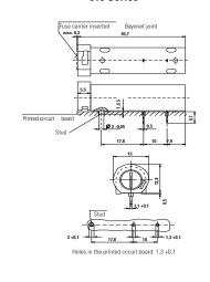
Fuse carrier inserted
