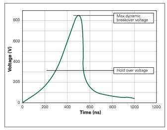
Note: Tested per 1kV/µs waveform
