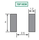
Recommended Soldering Pad Layout
