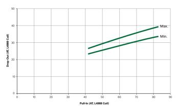
Note: Chart represents the range of Drop-Out, min to max for a given Pull-In value.
