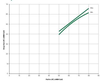
${\tt Note: Chart\ represents\ the\ range\ of\ Drop-Out,\ min\ to\ max\ for\ a\ given\ Pull-In\ value.}$
