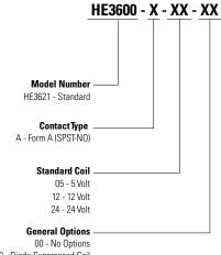
00 - No Options 10 - Diode Suppressed Coil 40 - External Magnetic Shield 50 - Ext. Magnetic Shield & Diode
