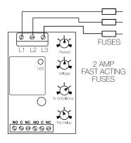
L1, L2, L3 = Line Voltage Input NO = Normally Open Contact NC = Normally Closed Contact C = Common, Transfer Contact
