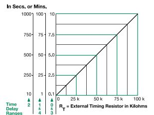
This chart applies to externally adjustable part numbers. The time delay is adjustable over the time delay range selected by varying the resistance across the RT terminals; as the resistance increases the time delav increases
