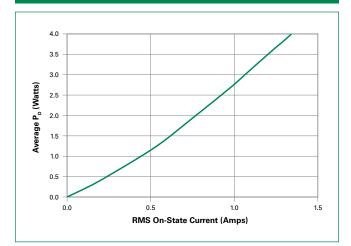
Figure 5: Pulse On-State Current Rating
