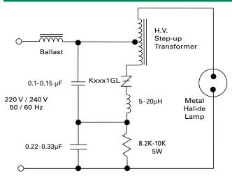
Note: With proper component selection, this circuit will produce three pulses for ignition of metal halide lamp that requires a minimum of three pulses at 5kV magnitude and >1uSec duration each at a minimum repetition rate of 3.3kHz.
