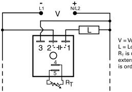
V = VoltageL = Load  $R_{\tau}$  is used when external adjustment is ordered.
