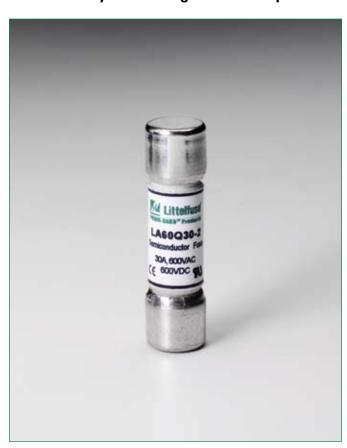
Littelfuse LA60Q semiconductor protection fuses feature a 600 volt AC/DC rating in a compact size (1½" x 13/32"). LA60Q also has the lowest I2t of all similar fuses and excellent cycling ability. Applications include inverters and small equipment requiring extremely fast response to faults, without the need to carry sustained heavy overloads.
