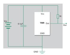
Note: It is strongly recommended that an external bypass capacitor be connected in-close-proximity to the device between the supply and ground pins to reduce noise. The recommended value for the external bypass capacitor is 0.1uf.
