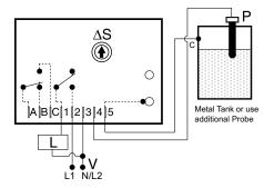
P = Probe L = Load V = Voltage  $\Delta S = Sensitivity$ Adjustment
