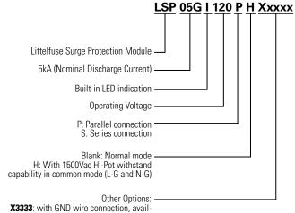
X3333: with GND wire connection, available for 240Vac and 277Vac rating with CE Marking for Class I earthed luminaire installation Wire Color: Line: Brown, Neutral: Blue, Ground/PE: Green with yellow stripe
