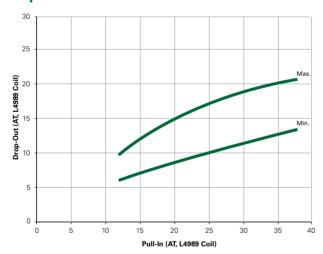
**Note:** Chart represents the range of Drop-Out, min to max, for a given Pull-In value of the MDCG-4 prior to modification into the MDSM-4.
