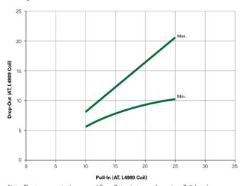
$\label{thm:continuous} \textbf{Note: Chart represents the range of Drop-Out, min to max for a given Pull-In value.}$
