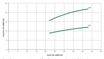
Note: Chart represents the range of Drop-Out,  $\min$  to  $\max$  for a given Pull-In value.
