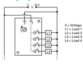
SC4 shown, For SC3, terminal 6 and load L4 are eliminated.
