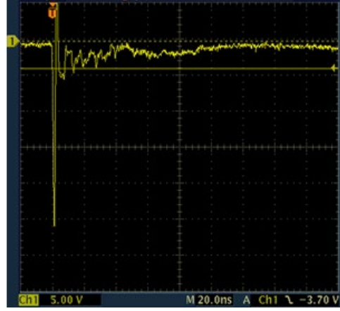
SP1124 IEC 61000 -4-2 -8 kV Contact ESD Clamping Voltage
