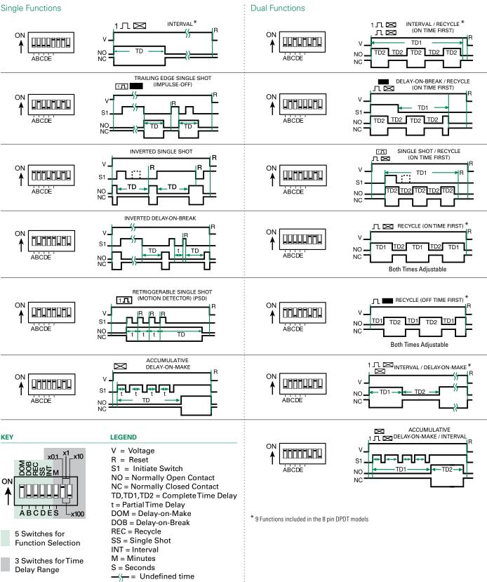
NOTE: The time delay range is the same for both functions when dual functions are selected.
