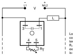
Load may be connected to terminal 3 or 1.  $R_{\rm T}$  is used when external adjustment is ordered.
