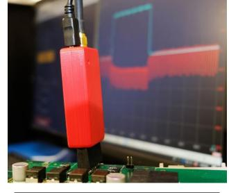
Note: For optimal performance when using a connector, ensure that the LoadSlammer<sup>TM</sup> is firmly seated and that the connector / blade are clear of debris. Failure to do so can result in unpredictable slewing behavior.
