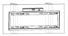
Install the wall plate to the wall
