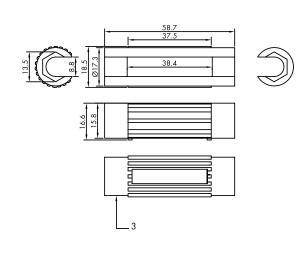
For stripping all common coax cables between 4.8 -7.5 mm dia. (e.g. for TV- and satellite antenna)
