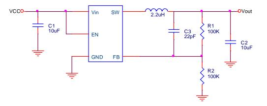
Adjustable Voltage Application Circuit
