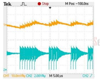
$CH_1 = \triangle V_{OUT}$ ,  $CH_2 = V_{SW}$  @  $V_{IN} = 3.7V$ ,  $V_{OUT} = 5V$ ,  $I_{OUT} = 1mA$
