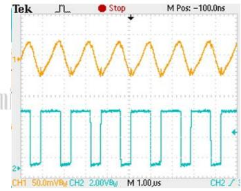
$CH_1 = \triangle V_{OUT}$ ,  $CH_2 = V_{SW}$  @  $V_{IN} = 3.7V$ ,  $V_{OUT} = 5V$ ,  $I_{OUT} = 500 mA$
