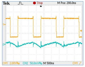
$V_{IN}$ =3.7V,  $V_{OUT}$ =5V,  $I_{OUT}$ =2A
