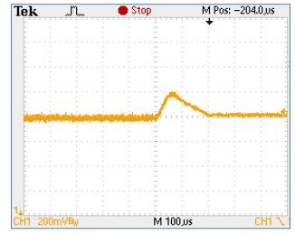
Output Unloading @ V<sub>IN</sub>=3V, I<sub>OUT</sub>=2A→0A
