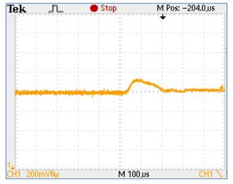
Output Unloading @ V<sub>IN</sub>=3.7V, I<sub>OUT</sub>=2A→0A
