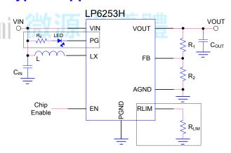
Note:  $C_{\text{OUT}}$  must be as close as possible to the PGND and VOUT pins.
