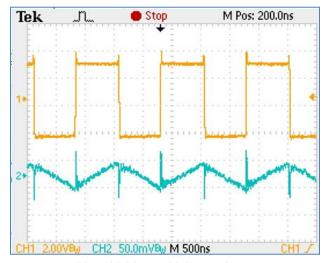
$V_{IN}$ =3V,  $V_{OUT}$ =5V,  $I_{OUT}$ =2A
