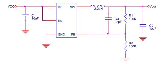
Adjustable Voltage Application Circuit
