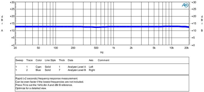
A-A FREQ RESP FAST @ 4ohm PO=4.8W CLASS AB VDD=6V.ats2
