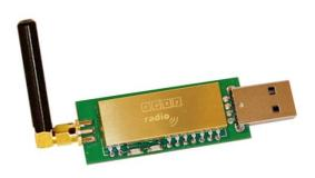
Utilising proprietary LPRS easyRadio technology operating in the 433MHz or 868MHz (UK & Europe) & 915MHz (US) Industrial Scientific & Medical (ISM) bands the eRA USB 'dongle' provides a simple 'wireless bridge' between any host devices that support USB serial communications such as a PC or Raspberry Pi or Beaglebone Black.
