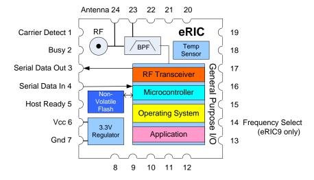
Figure I eRIC Transceiver Block Diagram
