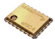
The easy Radio Intelligent Controller (eRIC) radio transceiver module is based on the Texas Instruments CC430F5137 System-on-Chip device to provide an intelligent radio sub-system that combines a high performance RF transceiver, RF band pass filters (BPF), an MSP430 microcontroller, 32Kb flash memory, non-volatile flash storage, temperature sensor, and a low drop voltage regulator. The device operates on the International licence exempt Industrial, Scientific and Medical (ISM) radio bands.
