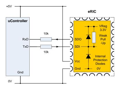
Figure 3 Connection to Host UART and I/O Protection
