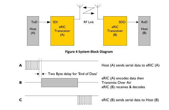
Figure 5 Timing Diagram
