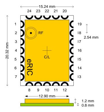
Figure 2 Mechanical Drawing
