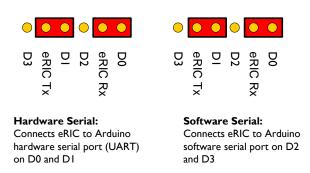
**Other Serial:** Alternatively remove the shorting jumpers and use male to female jumper wires. Connect the female ends of jumper wires to eRIC Rx and Tx pins and connect the male end to corresponding/preferred serial-enabled pins on Arduino<sup>M</sup>.
