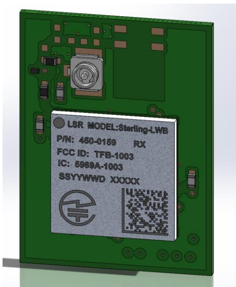
Figure 2: Sterling-LWB U.FL module (450-0148)
